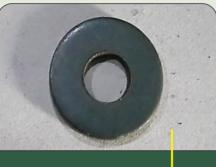
8mm Orifice (Reducer) Install in Ptg. Blanket Wash Line
