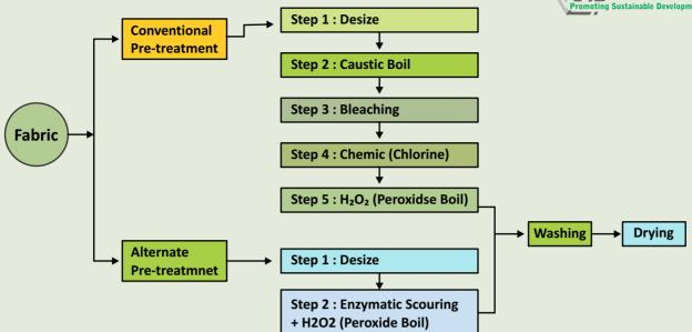
It can be observed that enzymatic scouring involves a smaller number of steps, consumes less time, power, and fuel, and reduces the overall cost.
